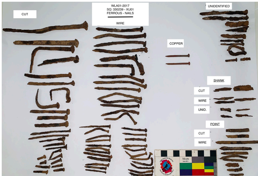
Figure 11.15. Range of nail types at the settlement (largely from Square 330239), including ferric cut, hand wrought and wire nails. Two copper nails, possibly from ship part.
